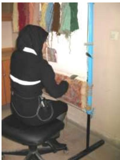
**Fig. 2:** Workstation B representing ergonomically designed carpet weaving based on current study (weaving height was 3 cm above elbowing height and 0° forward-sloping seat)
