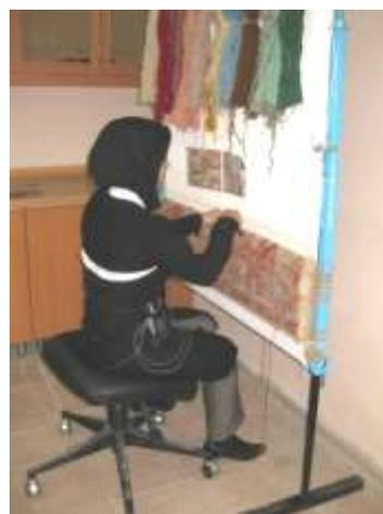
**Fig. 1:** Workstation A representing ergonomically designed carpet weaving based on previous studies (weaving height was 20 cm above elbow height and 10° forward-sloping seat)
