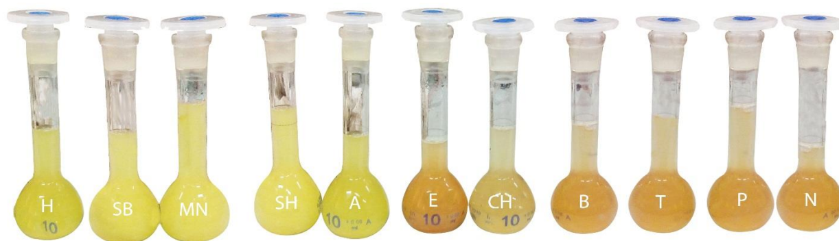
Figure 1. Results of colorimetric analysis of fresh lime juice (N) and products P, T, B, CH, E, A, SH, MN, SB and H using Ehrlich's reagent.
