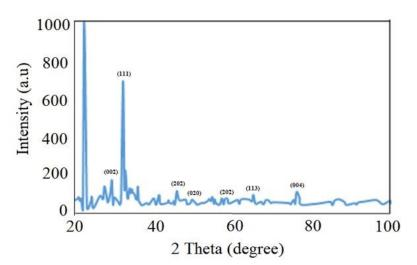
Figure 4. X-ray diffraction spectrum of CuO NPs synthesized from 0.1 M of CuSO<sub>4</sub> treated *Bacillus* sp. FU4 cell free supernatant at 28°C.
