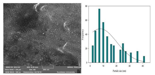
Figure 5. Scanning electron microscopy (SEM) image and particle size distributions of CuO NPs produced by culture supernatant of *Bacillus* sp. FU4.
