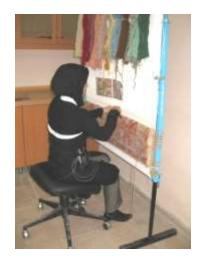
**Fig. 1:** Workstation A representing ergonomically desingned carpet weaving based on previous studies(weaving height was 20 cm above elbow height and10° forward-sloping seat)
