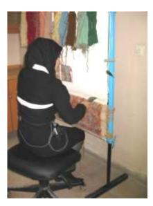
Fig. 2: Workstation B representing ergonomically desingned carpet weaving based on current study(weaving height was 3 cm above elbowing height and 0° forward-sloping seat)
