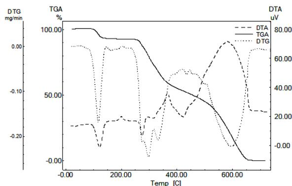
Figure 2. TGA, DTG and DTA curves of TER.
